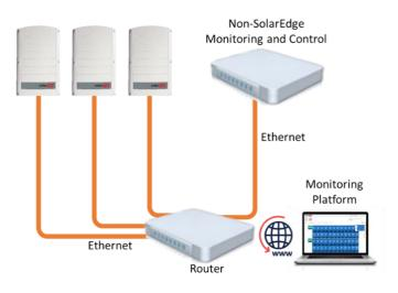
Option 2 – Connect the Leader only to the Ethernet router via Ethernet cables.
