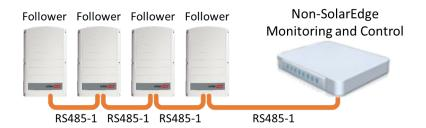
Option 2 – Use RS485-1 to connect Follower inverters to the Leader; use either RS485-2 or RS485-E to connect the Leader to a non-SolarEdge monitoring device. Every inverter in the
