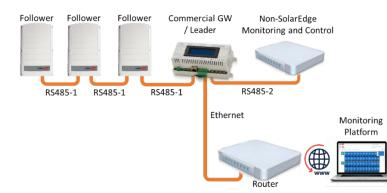
If required, use the RS485-E bus for connecting a second chain of inverters.
