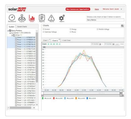
The chart view from the SolarEdge monitoring platform shows the performance of individual panels. This graph illustrates that the power of each panel is optimal and independent of other panels in the same string. The dips show the effects of roof level obstructions.
