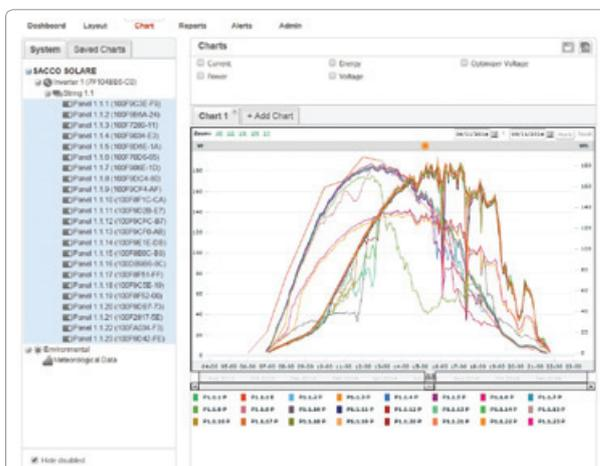
The Chart view from the SolarEdge monitoring portal shows the performance of every individual module. This screenshot shows how modules in the same string placed on different orientations perform independently of each other.
