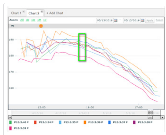
Figure 10b: Power curves demonstrate 7% mismatch between best and worst Modules at 4pm
