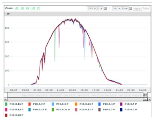
Figure 5: Power curves demonstrate transient shading patterns on individual modules, implying dynamic cloud fronts partially covering the array
