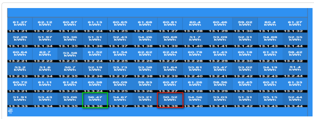
Figure 9: Layout yearly view shows the mismatch in energy production between modules in the same string
