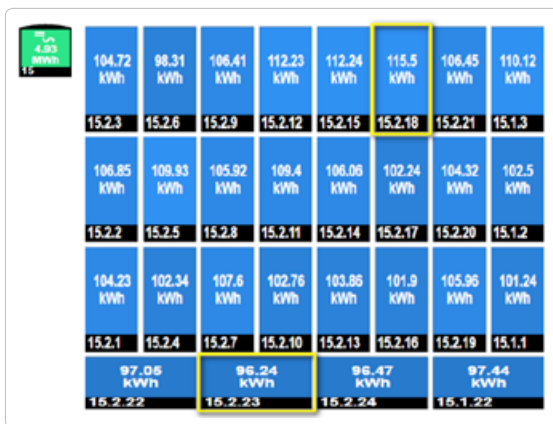
Figure 1: Layout view showing yearly energy production for string 15.2. Significant mismatch between adjacent modules and modules in the same string is observed
