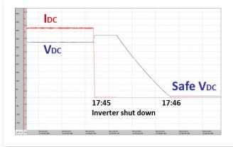
This graph represents an automatic string shutdown. As demonstrated, the current is shut down immediately once AC power or Inverter is turned off. The string voltage is reduced to safe voltage in 180 seconds.
