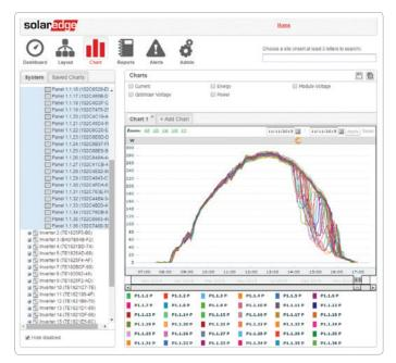
The chart view from the SolarEdge monitoring portal shows the performance of individual modules. This graph illustrates that the power of each module is optimal and independent of other modules in the same string. The dips show the effects of inter-row shading.
