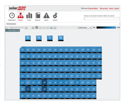
the maintenance staff on the exact location of modules requiring, for example, cleaning.
