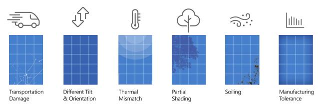
With traditional inverters, the weakest module reduces the performance of all modules in a string. With SolarEdge, each module produces the maximum energy, and power losses are minimised.
