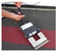
**2** Loop the module wire leads through the bracket to manage the excess wire.
