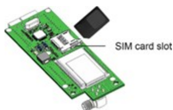
Figure 23: Inserting the SIM card into the GSM modem
