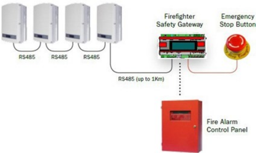
Figure 2: Example of SolarEdge firefighter gateway connections
