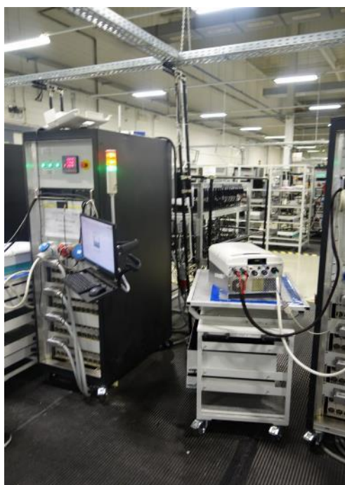
Figure 5-11 SolarEdge Inverters Undergoing Manufacturing Test
