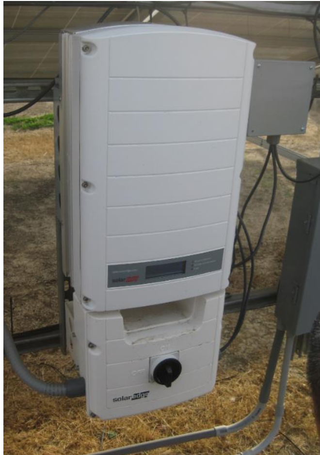
Figure 9-14 SE20KUS (480 VAC, 3-phase) Inverter Under Test
