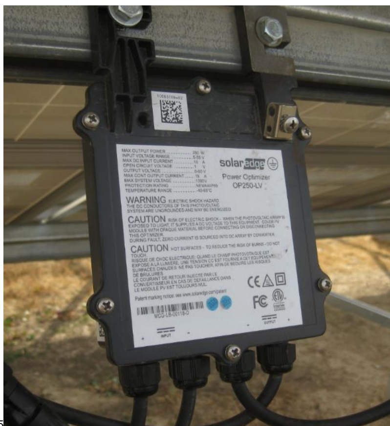
Figure 9-13 OP 250-LV Optimizers Under Test
