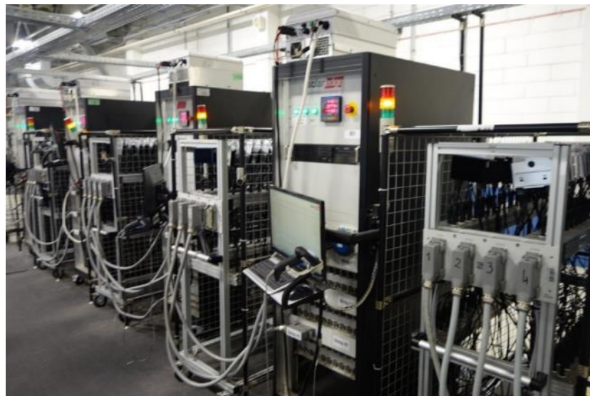
Figure 5-9 Optimizers Undergoing Integrative Testing
