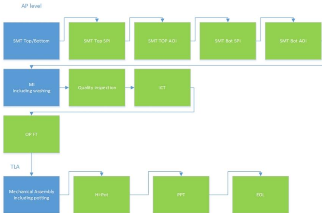
Figure 5-2 SolarEdge Optimizer Manufacturing Test Steps
