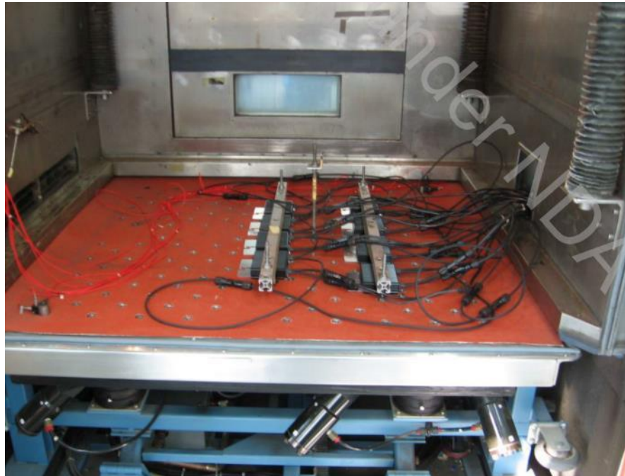
Figure 4-11 SolarEdge power optimizers in HALT test chamber
