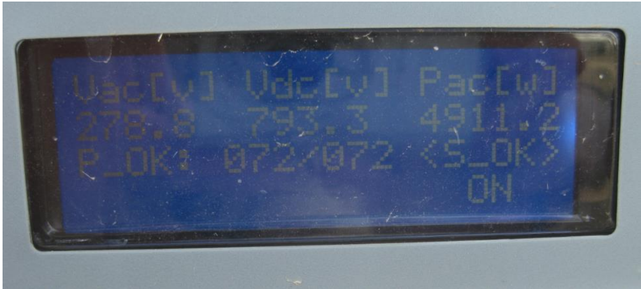
Figure 9-15 Photo of Inverter LCD Showing Operating Parameters
