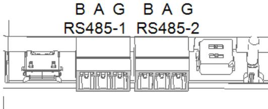
Figure 13: Data Logger RS485 connectors and termination switches
