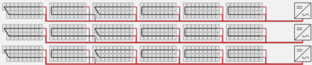
SolarEdge cabling diagram | Total of 27 strings
