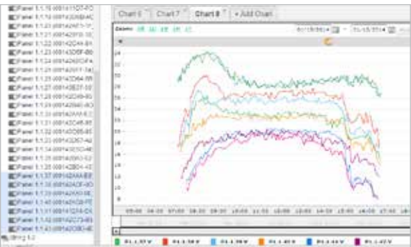
No need to send technicians to the roof –panel voltage is measured remotely
