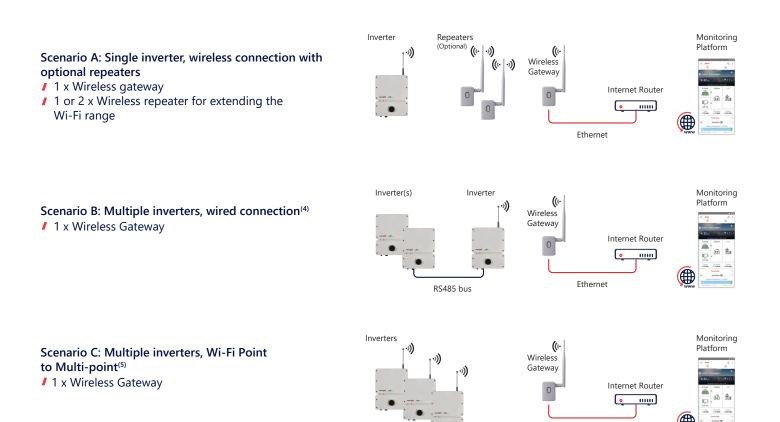
(4) To extend the Wi-Fi range, add one or two Wireless Repeaters(5) Additional inverter antennas should be purchased separately
