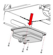
Remove the communications board assembly
