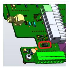
8. Guide the holes in the communications board assembly over the two guide pins. Make sure you don't bend or trap the cables.
