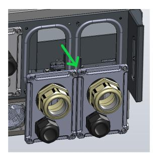
Removing the AC Plate
