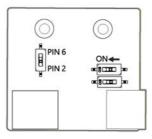
Figure 17: DIP switch set-up on the CAN board
