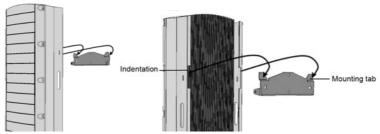
Figure 7: Hanging the inverter on the bracket
