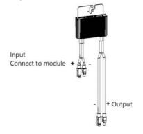
Figure 3: Power optimizer connectors
