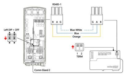
Figure 14: Meter Connection 2
