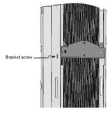
Figure 8: Inserting the bracket screws
