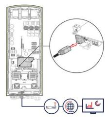
Figure 21: RJ45 Ethernet connection
