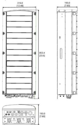
Figure 25: StorEdge Three Phase Inverter dimensions
