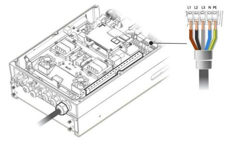
4. Open the AC gland and insert the AC cable through the gland.
