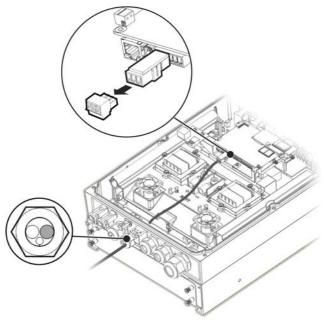
Figure 13: Meter Connection
