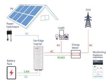
Figure 1: StorEdge system components
