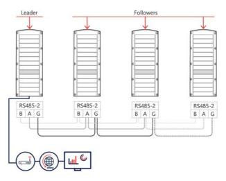
Figure 23: Connecting the inverters in a chain
