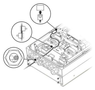
Figure 16: Connection of CAN Cable from Battery to Inverter
