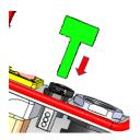
2. Re-connect the LED indicator cable to the LED board. Pull the connector gently to make sure it is properly connected.
