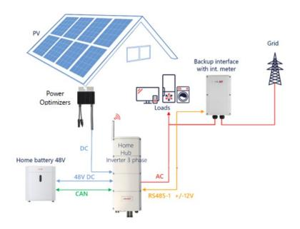
In a PHB configuration, some home appliances are connected on the load side of the BUI. These appliances operate during backup if the load's power consumption meets the design guidelines.
