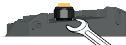
Fig. 6-14: Tighten the cable gland from the back
