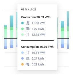
In **energy** mode, the aggregated production and/or consumption for each time interval is displayed. When looking at multi-day energy, the weather icon refers to the on-site weather conditions reported at noon.
