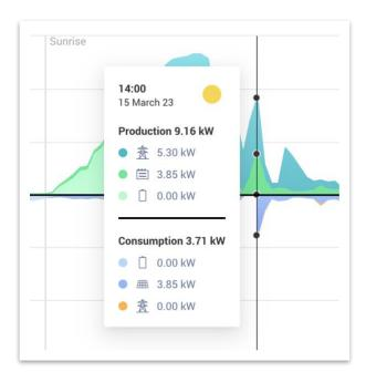
Hovering over a specific point displays a detailed view of production and consumption at that time. In supported sites, **energy sources and destinations** for the data point are displayed. The weather icon indicates the site weather conditions, as reported by our weather service partner at that time.
