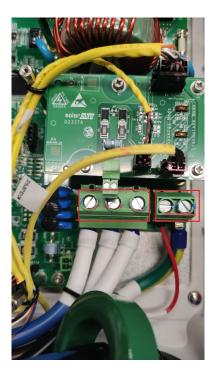
4. Disconnect the AC cable from the AC plug.
