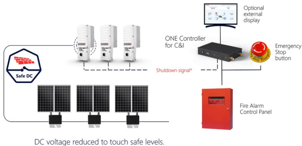
Figure 1: FFG attached to the ONE Controller C&I diagram
