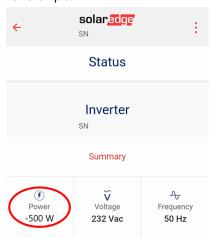
This only happens when your StorEdge inverter charges the battery from the AC grid, and not from PV modules, as it normally does. In this case AC power from the gird is converted into DC power, and a negative power value is displayed in SetApp.
