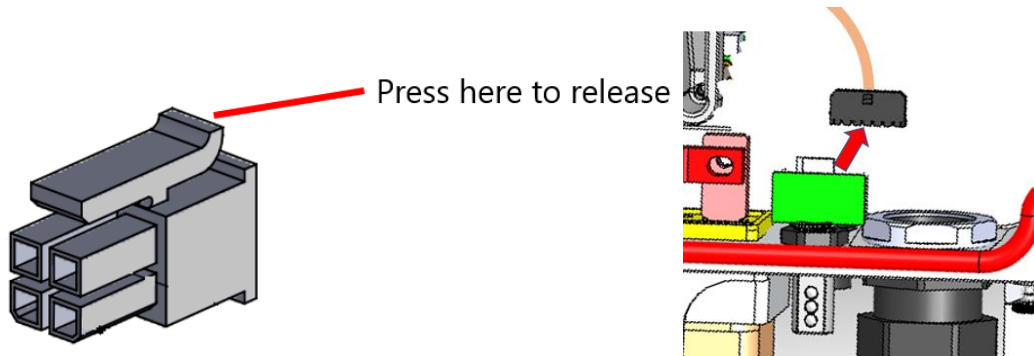
Figure 3: remove LED cable connector
