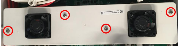
Figure 3: remove Internal Fans assembly
