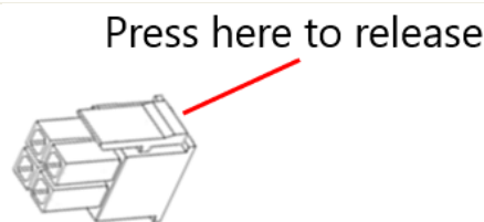
Figure 4: connector locking mechanism
