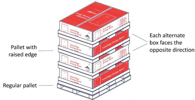
Figure 1: Pallet Packed with a Maximum of Four SolarEdge Home Batteries Boxes for Shipping
