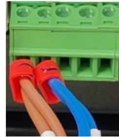
7. Pull out the wires from the 10-pin green connector.
