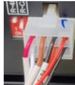
2. Reconnect the wires of the 5-pin green terminal cable.
