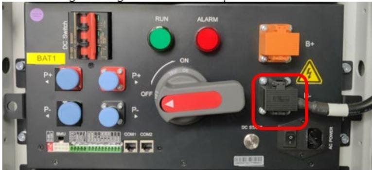
4. Repeat the same steps to reattach the orange cable to its terminal block.
