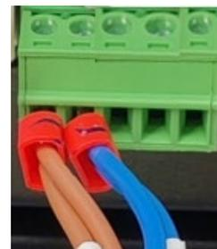
3. Reconnect the wires of the 10-pin green terminal cable.
