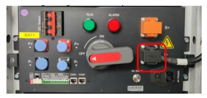
6. Repeat the same steps to reattach the orange cable to its terminal block.
