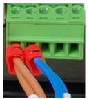
3. Reconnect the wires of the 10-pin green terminal cable.
