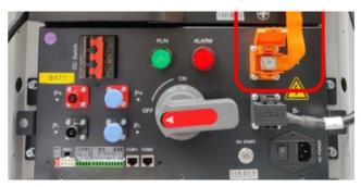
11. Use a 13mm socket and a wrench to remove the bolt securing the soft copper cable.
