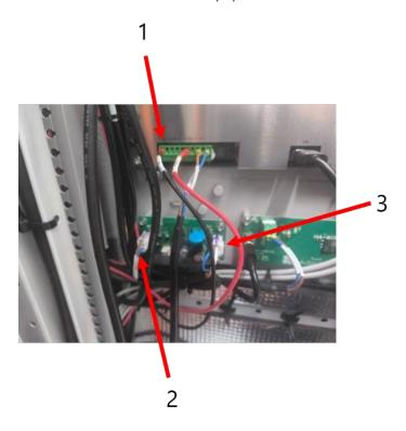
4. Using a Philips screwdriver, loosen the four screws on the auxiliary power board.
