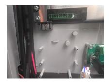
6. Align and place the new auxiliary power board on the standoffs.
