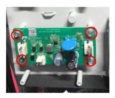
5. Remove the old auxiliary power board from the standoffs.
