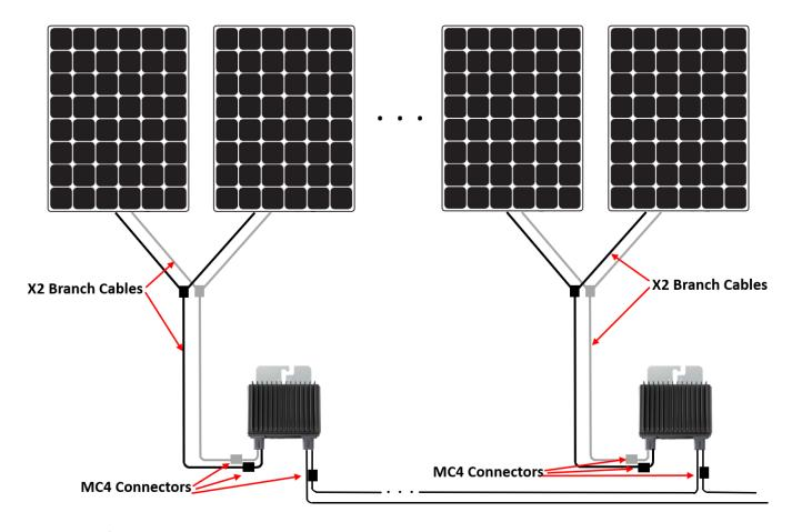
Sense Connect feature supported only at the MC4 connectors at the Power Optimizers short cables.
