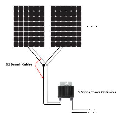
Two (2) Branch Cables connecting two (2) PV Modules to an S-Series Power Optimizer
