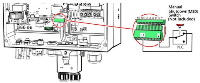
For more information on connecting the MSD switch to the SolarEdge Home Hub Inverter - Three Phase, refer to the SolarEdge Home Hub Inverter Three Phase Quick Installation Guide.
