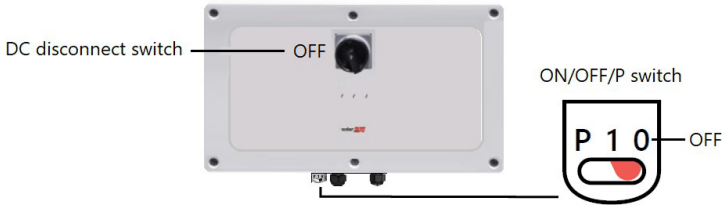
Figure 31: Synergy Manager ON/OFF/P and DC disconnect switches
