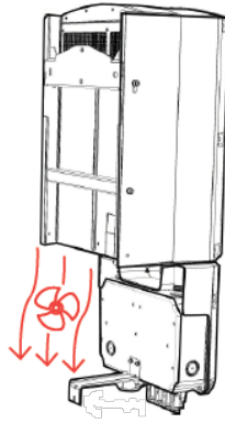
Figure 16: Inverter fan - airflow
