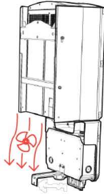
Figure 12: Inverter fan - airflow
