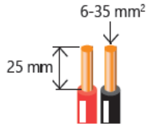
Figure 21: Stripping insulation from the DC wires
