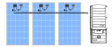
Figure 4: Power Optimisers connected in series
