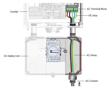
Figure 16: AC cable route inside the DC Safety Unit and inverter
