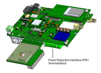
Figure 32: PRI Terminal Block Location on the Communication Board of the Inverter For detailed connection and configuration of the inverter in alternative power source mode, refer to: <u>https://www.solaredge.com/sites/default/files/se-inverter-support-of-</u>voltage-sources.pdf
