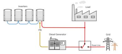
Figure 31: Example of Alternative Power Source System
