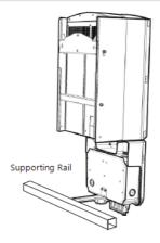
Figure 11: Supporting rail on the back of the DC Safety Unit
