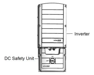
Figure 5: Inverter front view
