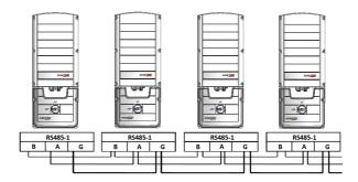
Figure 29: Connecting the inverters in chain
