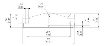
Figure 34: Dimensions of Inverter mounting bracket
