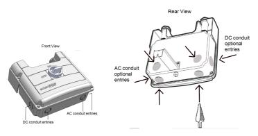
Figure 9: DC Safety Unit conduit entries
