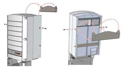
Figure 13: Hanging the inverter on the brackets
