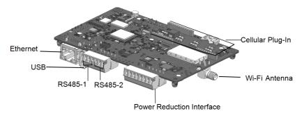
Figure 23: Internal communication connectors
