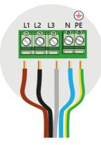
Figure 18: Connecting wires to the terminal block
