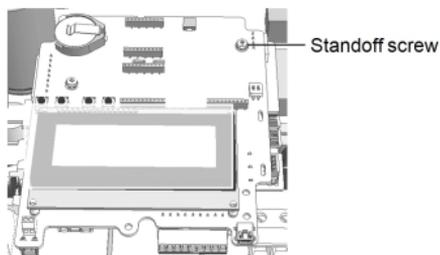
Figure 13: The communication board
