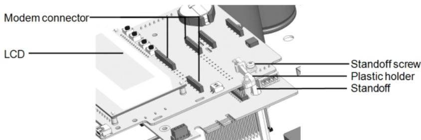
Figure 14: The holder installed on the communication board
