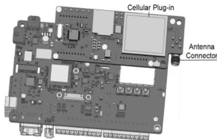
Figure 1: Communications Board with Cellular Plug-in
