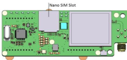
Figure 7: Nano SIM card slot on Cellular Plug-in
