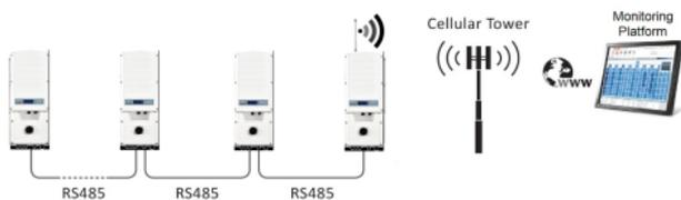
Figure 9: Cellular Plug-in Connection Diagram - Commercial Installation
