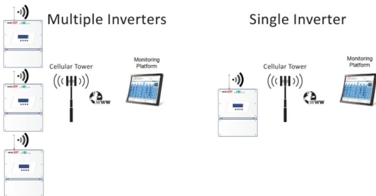
Figure 8: Cellular Plug-in Connection Diagram - Residential Installation
