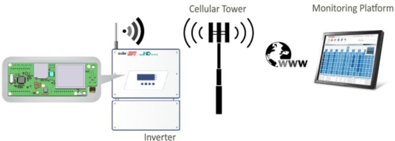
Figure 2: Connecting the Inverter to the Monitoring Platform
