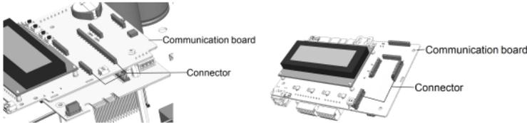
Figure 5: Communication board with Cellular connector
