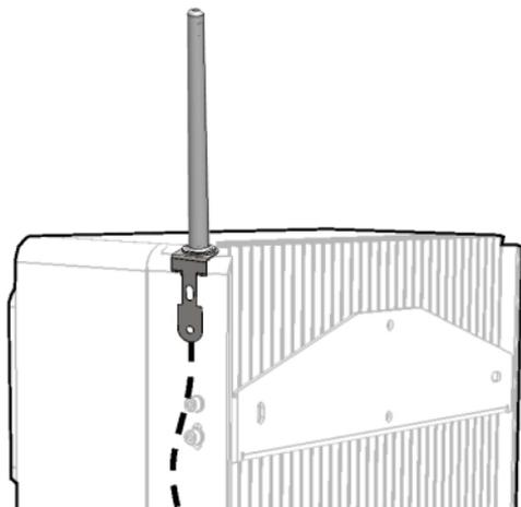
Figure 10: Routing the antenna cable
