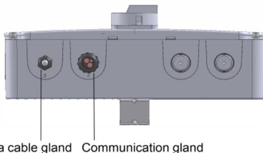
Figure 11: Connection via antenna cable gland
