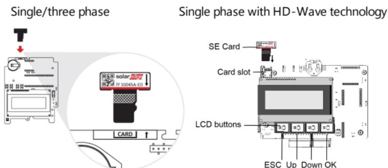
Figure 6: Communication board and activation card
