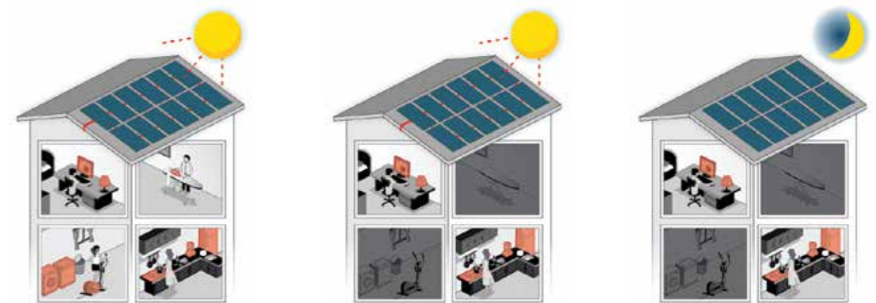
Charge battery from the PV system
