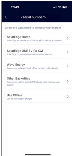
5. On the **<serial number>** screen, select **SolarEdge Home**. This connects to SolarEdge residential installations with an inverter on-site.
