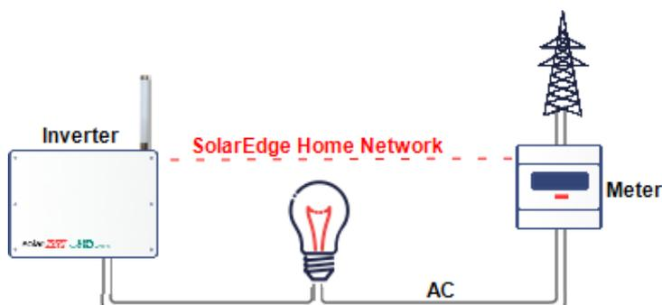
Figure: Single-inverter connection with inline meter over SolarEdge Home Network
