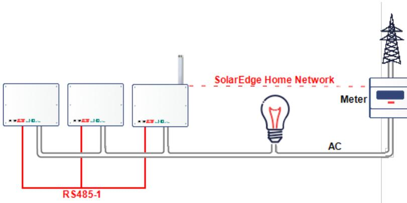
Figure : Multi-inverter System SolarEdge Home Network Meter
