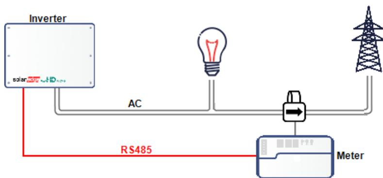
Figure: Single-inverter connection with RS485 meter
