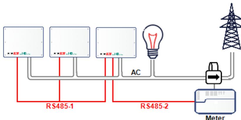
Figure: Multi-inverter connection with inverter as Smart Energy Manager
