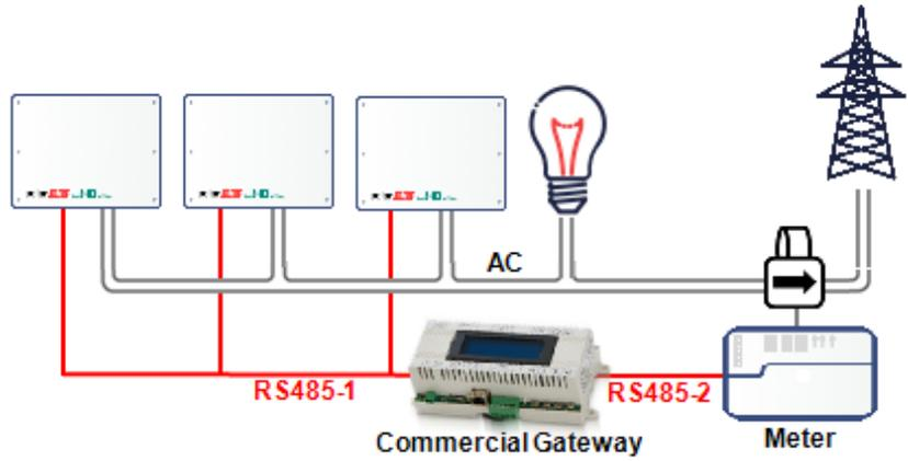
Figure: Multi-inverter connection with Commercial Gateway
