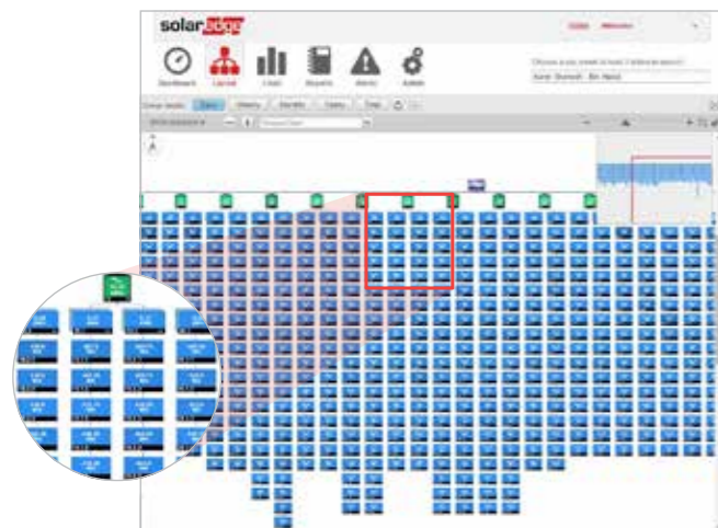
The logical layout displays the electrical connectivity between panels, strings and inverter
