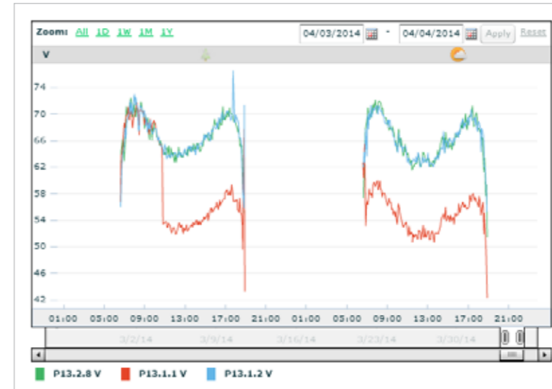
It is easy to identify the bypass diode failure with the panel-level voltage graphs. The faulty panel outputs at only 2/3 of the voltage (5/6 in this case of power optimiser connected to two panels).
