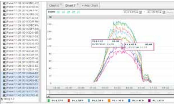
Looking at the modules within one string, it is possible to see the power degradation increasing towards the negative pole.
