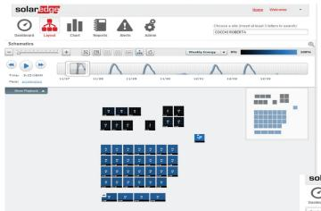
The Layout view from the SolarEdge monitoring portal shows the system's physical layout. The blue color code indicates the performance level of each module and proves that each module works in an individual capacity. In this case, darker modules are on the roof facet receiving less sunlight.
