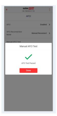
Inverter production is interrupted simulating a detected arc, and one of the following error codes displays:
