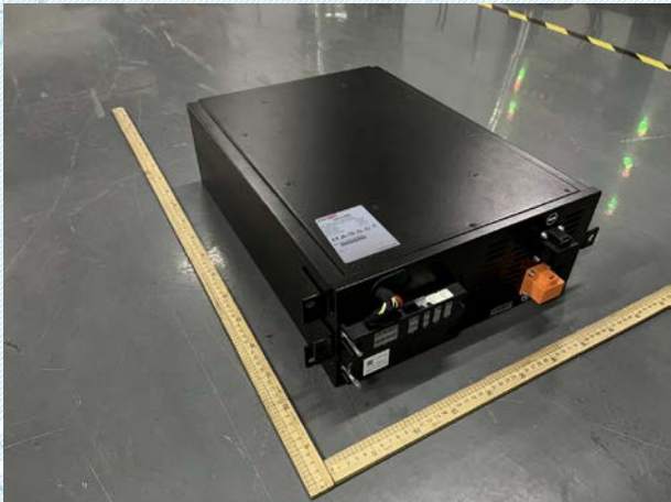
Battery module appearance 电池模组外观
