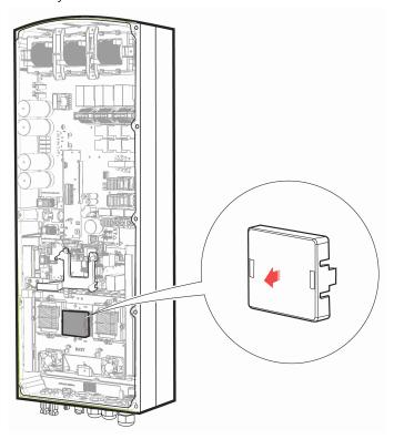
2. Release the screw that fastens the MC4 cable tunnel cover (Screw 1) and the remove cover.
